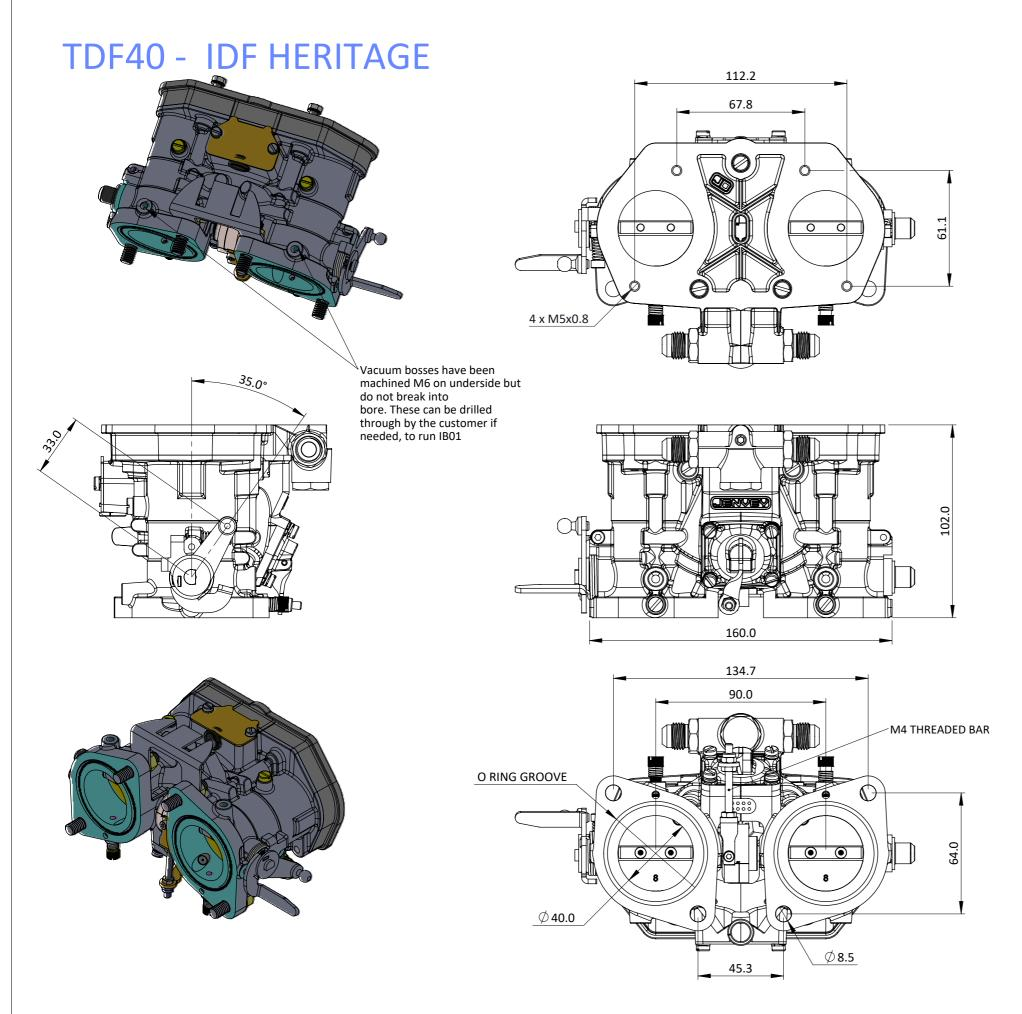
The Heritage body is designed with major dimensions identical to twin vertical carburettors from Weber, Dellorto, Solex etc. The fuel rail is integrated within the body lid, supplied with Bosch injectors.
