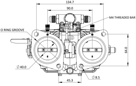
The Heritage body is designed with major dimensions identical to twin vertical carburettors from Weber, Dellorto, Solex etc. The fuel rail is integrated within the body lid, supplied with Bosch injectors.
