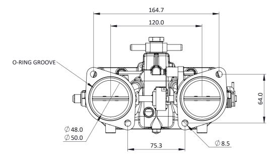
The Heritage body is designed with major dimensions identical to twin vertical carburettors from Weber, Dellorto, Solex etc. The fuel rail is integrated within the body lid, supplied with Bosch EV14 730cc/min injectors.
