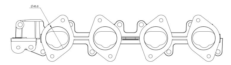
MAY BE PORTED OUT TO 50MM AT BODY FLANGE AND PROPORTIONALLY AT HEAD FLANGE. BOSSES ON UNDERSIDE FOR VACUUM TAPPINGS.
