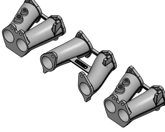
NISSAN DATSUN L28 MANIFOLD SET FOR 240Z, 260Z, 280Z, 280ZX. THE SET OF MANIFOLDS FITS TO THE DATSUN L-SERIES 6 CYLINDER ENGINES (L28. WILL ALSO FIT L26, L24) AND HAS BEEN PORTED TO MATCH 50mm THROTTLE BODIES AT THE INLET (WHICH CAN BE PORTED UP TO 55mm) AND 40mm ON THE CYLINDER HEAD SIDE AND CAN BE USED WITH ANY DCOE STYLE FLANGE THROTTLE BODY.
