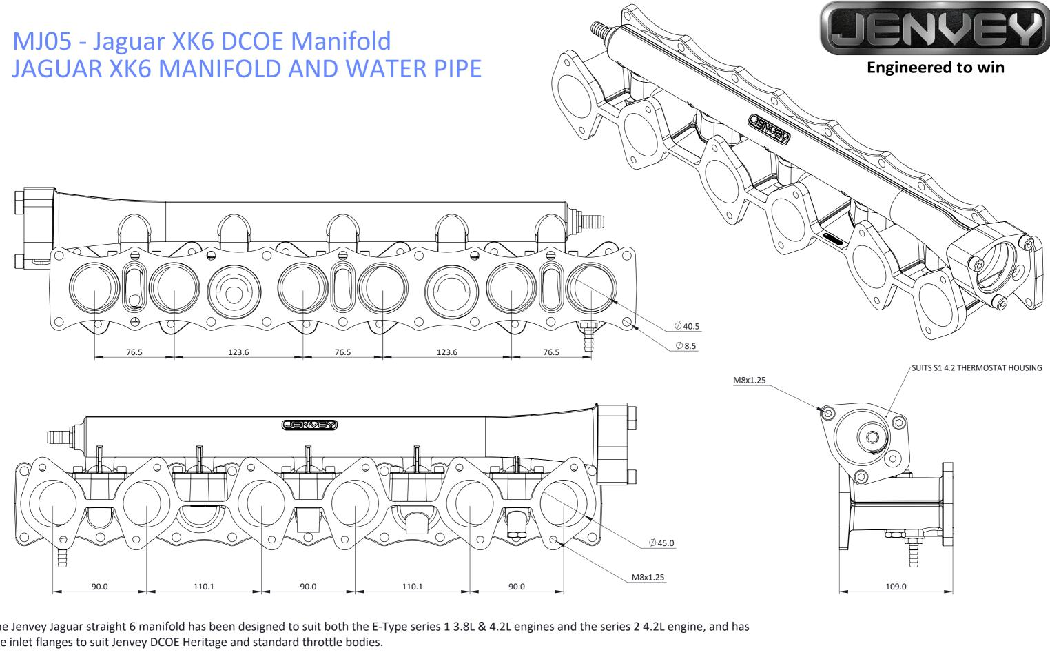
The Jenvey Jaguar straight 6 manifold has been designed to suit both the E-Type series 1 3.8L & 4.2L engines and the series 2 4.2L engine, and has the inlet flanges to suit Jenvey DCOE Heritage and standard throttle bodies.
