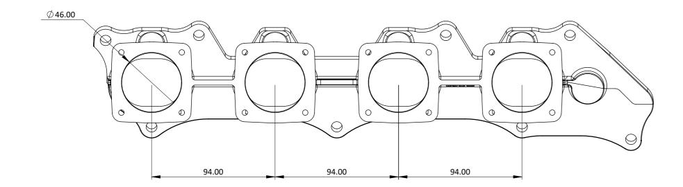
FLANGES FOR JENVEY SF THROTTLE BODIES. MAY BE PORTED OUT TO 52mm AT BODY FLANGE AND PROPORTIONALLY AT HEAD FLANGE. UNDRILLED BOSSES ON TOP SIDE FOR INJECTOR PORTS, VACUUM TAPPINGS ETC. UNDRILLED BOSSES ON UNDERSIDE VOR VACUUM TAPPINGS.
