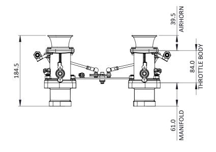
AN INDIVIDUAL THROTTLE BODY KIT FOR THE JAGUAR V12 WHICH CONTAINS A SET OF SIX INLET MANIFOLDS, SIX 40mm 40TFSF THROTTLE BODIES AND 40mm LONG HERITAGE AIRHORNS.
