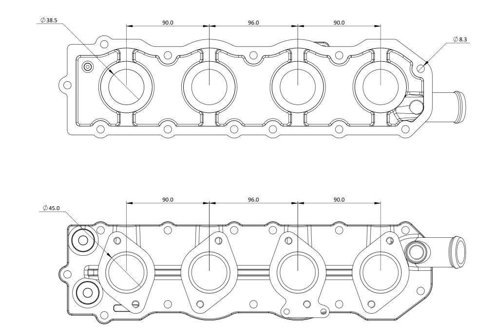
MADE FOR 105 T/SPARK CONVERSIONS, MANIFOLD BOLTS STRAIGHT ON TO A STD 2.0 TWIN SPARK ALFA 75 ENGINE AND EARLY 164 ENGINES AND CAN ALSO BE FITTED INTO 105 SERIES CARS.
