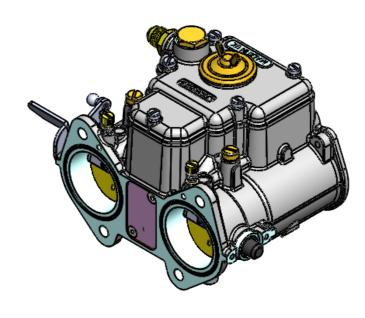
The Heritage body is designed with major dimensions identical to twin horizontal carburettors from Weber, Dellorto, Solex etc. The fuel rail is integrated within the body lid, supplied with Bosch EV14 350cc/min injectors.
