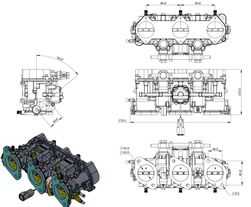
The Heritage triple body is designed with major dimensions identical to triple vertical carburettors from Weber.
