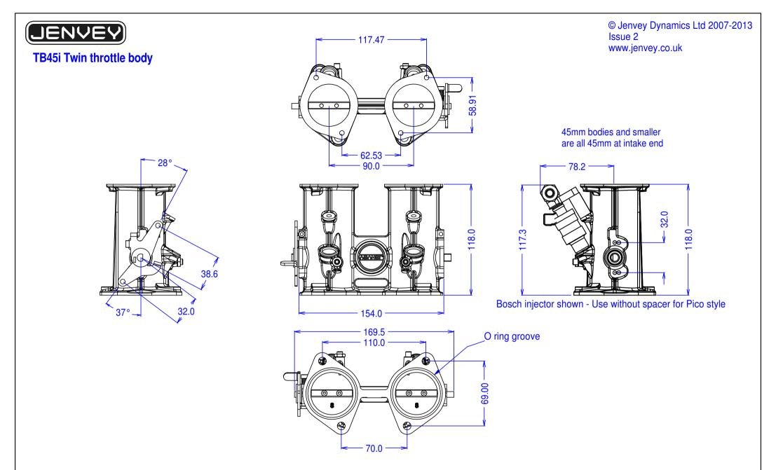
The TB body is designed with major dimensions identical to twin horizontal carburettors from Weber, Dellorto, Solex etc. and finished in crackle black powder coat. The fuel rail (supplied seperately) fits within the length of the body with either Pico and Bosch style injectors, allowing use of a flat airfilter backplate. The body comes with 'O' rings on the outlet, idle bypass adjustment, interconnecting link and bungs for the inlet end.
