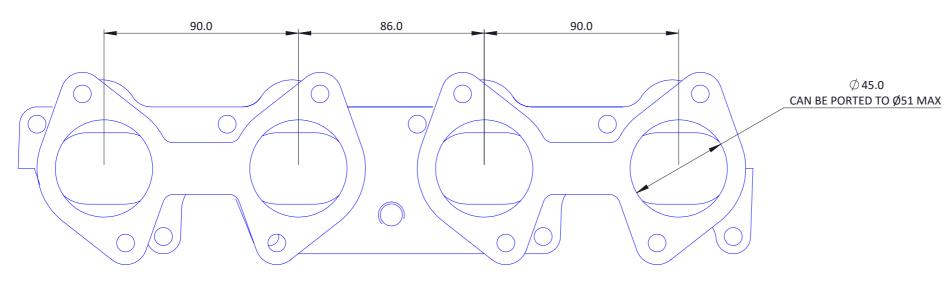
MANIFOLD TO FIT VOLKSWAGEN 2.0L 16V ENGINE SUCH AS THE OLDER 1.8 AND 2.0 SHORT AND TALL BLOCK ENGINES INCLUDING KR 9A ABF PL AS USED IN GOLFS, SCIROCCOS AND BORAS.
