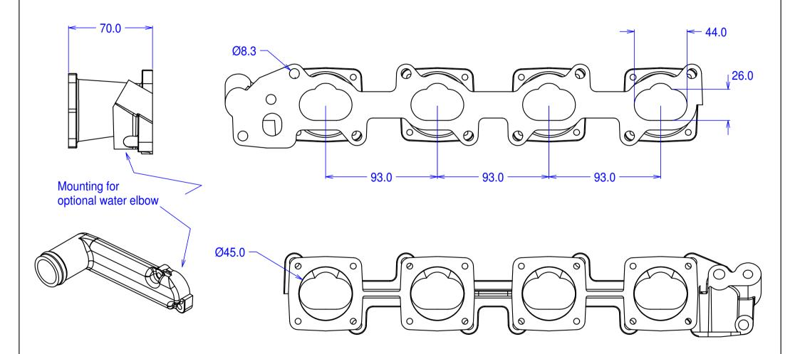
Flanges for Jenvey SF throttle bodies. May be ported out to 50mm at body flange and proportionally at head flange. Bosses on underside for vacuum tappings.
