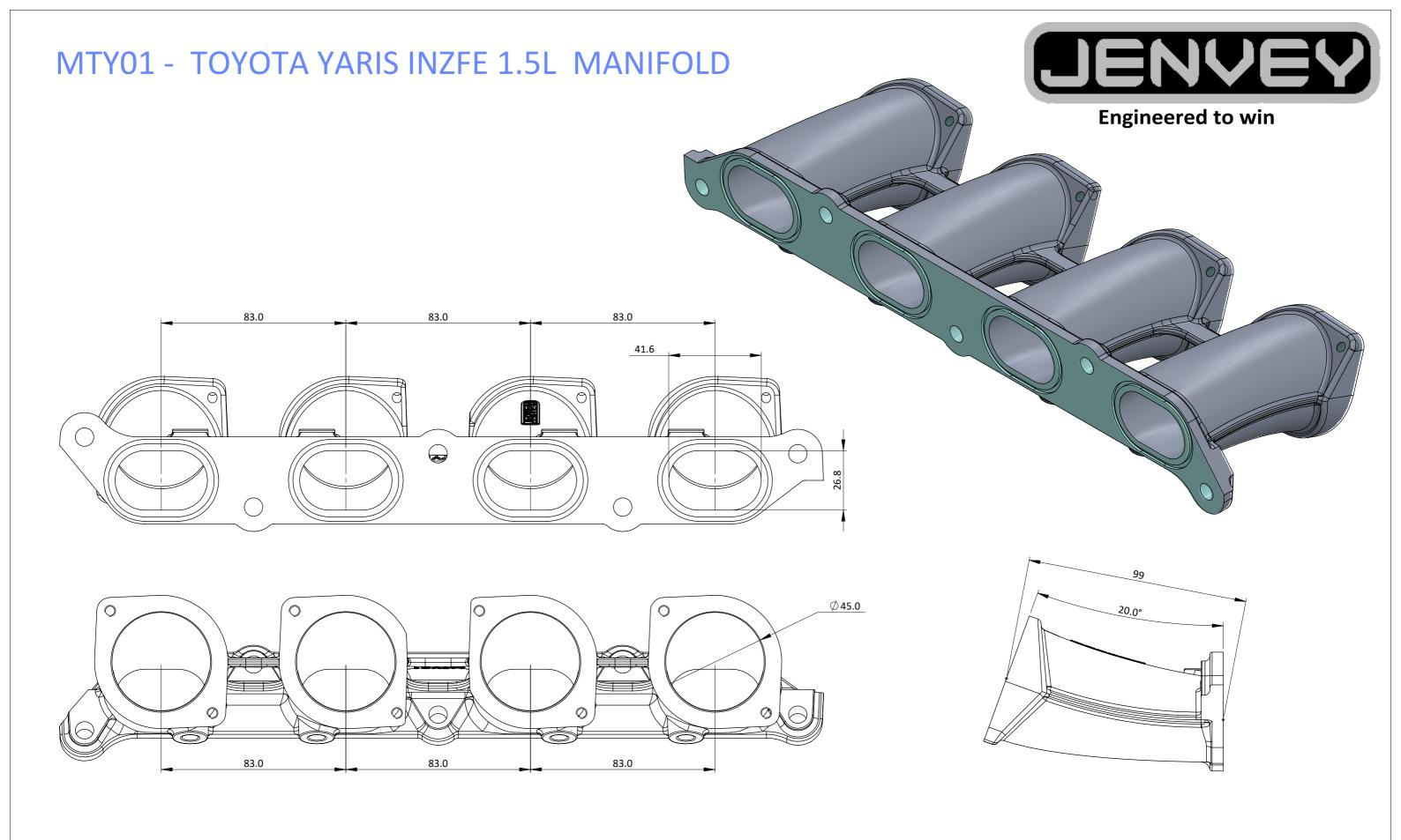
Inlet manifold for ST throttle bodies to fit a Toyota Yaris 1.5 litre. Ø45mm inlet, can be ported to head. Includes extra undrilled bosses on the side for idle air / vacuum take off / etc.
