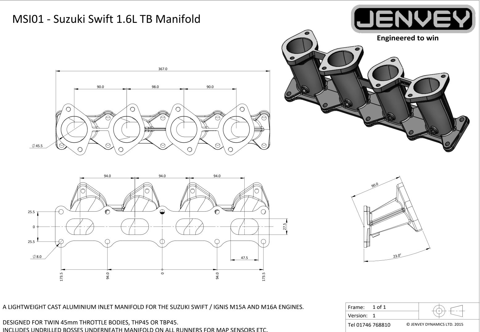
DESIGNED FOR TWIN 45mm THROTTLE BODIES, THP45 OR TBP45. INCLUDES UNDRILLED BOSSES UNDERNEATH MANIFOLD ON ALL RUNNERS FOR MAP SENSORS ETC.
