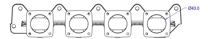
Flanges for Jenvey SF throttle bodies. May be ported out to 46mm at body flange and proportionally at head flange. Undrilled tapping bosses on underside for brakes, fast idle valve, sensors etc.
