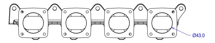
Flanges for Jenvey SF throttle bodies. May be ported out to 46mm at body flange and proportionally at head flange. Undrilled tapping bosses on underside for brakes, fast idle valve, sensors etc.
