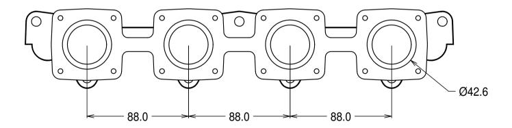
Flanges for Jenvey SF throttle bodies. May be ported out to 46mm at body flange and proportionally at head flange. Undrilled bosses on top side for injectors or brakes, fast idle valve, sensors etc.
