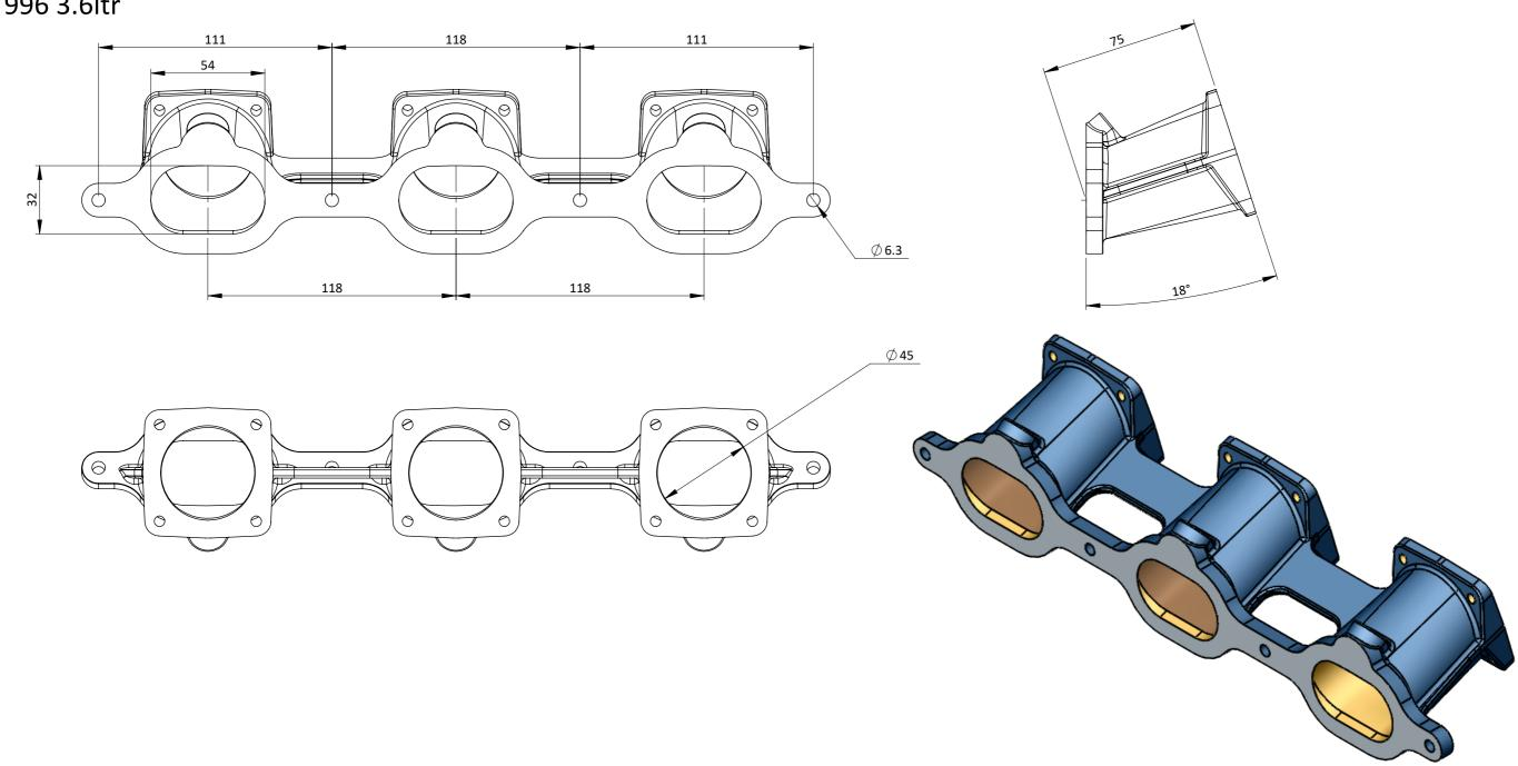
MAY BE PORTED OUT TO 50MM AT BODY FLANGE AND PROPORTIONALLY AT HEAD FLANGE.
