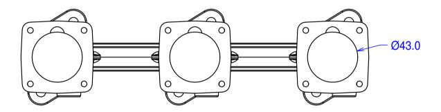
May be ported out to 46mm at body flange and proportionally at head flange. Bosses on each port for vacuum tappings. Compatible with standard cooling shroud.
