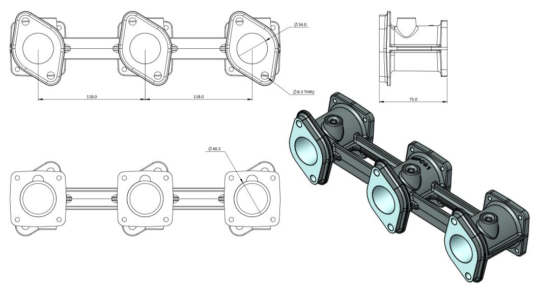
MAY BE PORTED OUT TO 46MM AT BODY FLANGE AND PROPORTIONALLY AT HEAD FLANGE.
