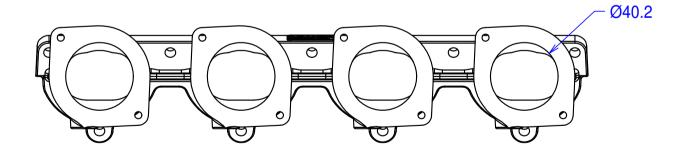
Flanges for Jenvey ST throttle bodies or SF with spindle mods. May be ported out to 45mm at body flange and proportionally at head flange. 2 bosses at ends and 4 on underside for vacuum tappings.
