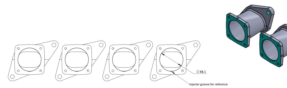
A set of 4 single stub manifolds to mount a set of individual SF throttle bodies to a Nissan 2L SR20VE High port engine. This will only fit certain models, not the DET version.
