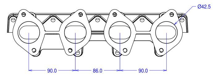
May be ported up to 46mm at body flange and proportionally at head flange. Undrilled bosses on top side for injector ports, vacuum tappings etc. and undrilled bosses on underside for vacuum tappings.
