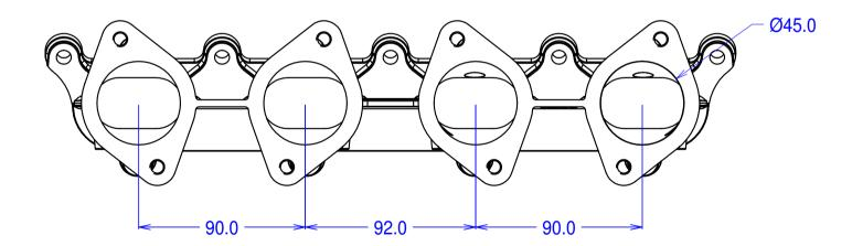
May be ported up to 50mm at body flange and proportionally at head flange.
