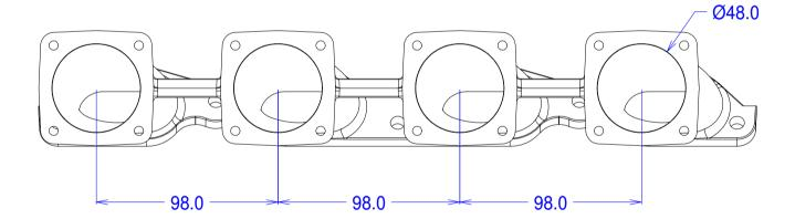
Flanges for Jenvey SF throttle bodies. May be ported up to 52mm. Additional material to allow matching to ported cylinder heads
