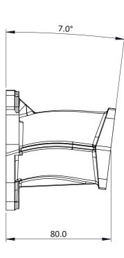
MAY BE PORTED OUT TO 52MM AT INLET FLANGE AND PROPORTIONALLY AT HEAD FLANGE.
