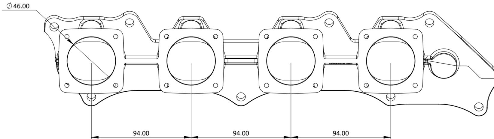
FLANGES FOR JENVEY SF THROTTLE BODIES. MAY BE PORTED OUT TO 52mm AT BODY FLANGE AND PROPORTIONALLY AT HEAD FLANGE.
