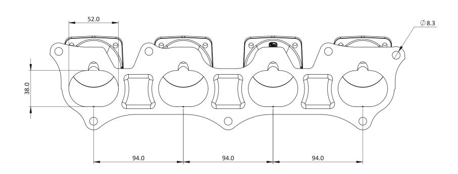
MAY BE PORTED OUT TO 52MM AT INLET FLANGE AND PROPORTIONALLY AT HEAD FLANGE. INDRILLED BOSSES ON TOP SIDE FOR INJECTOR PORT, VACUUM TAPPINGS ETC. UNDRILLED BOSSES UNDERNEATH FOR IDLE AIR, BRAKE TAPPING, SENSORS, ETC. NOW 15% LIGHTER WITH LIGHTENED HEAD FLANGE.
