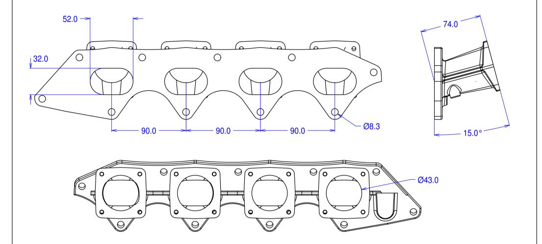
Flanges for Jenvey SF throttle bodies. May be ported out to 48mm. Undrilled bosses on underside for vacuum tappings.
