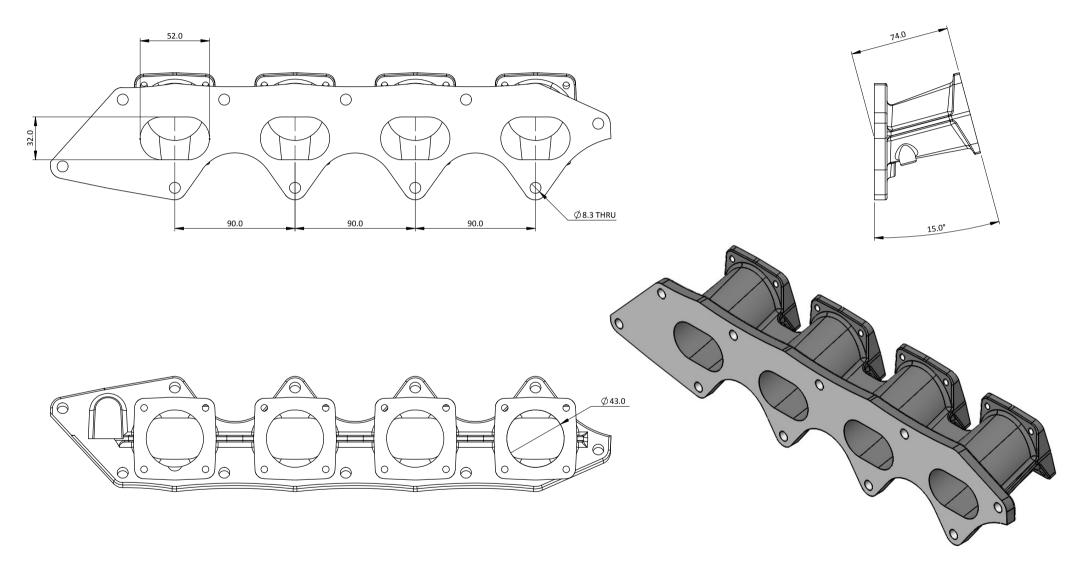
FLANGES FOR JENVEY SF THROTTLE BODIES. MAY BE PORTED OUT TO 48MM. UNDRILLED BOSSES ON UNDERSIDE FOR VACUUM TAPPINGS.
