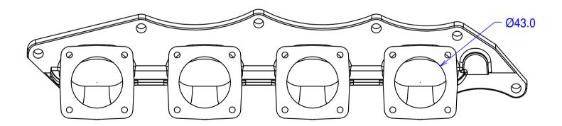
Flanges for Jenvey SF throttle bodies. May be ported out to 48mm. Undrilled boss for coolant tapping.
