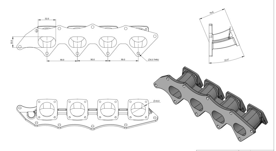
FLANGES FOR JENVEY SF THROTTLE BODIES. MAY BE PORTED OUT TO 48MM. UNDRILLED BOSS FOR COOLANT TAPPING.
