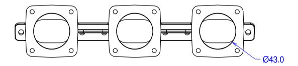
Flanges for Jenvey SF throttle bodies. May be ported up to 46mm at body flange and proportionally at head flange. Supplied as matched pair.
