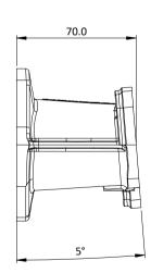
Flanges to suit Jenvey twin DCOE throttle bodies. May be ported up to 50mm. Additional material to allow matching to ported cylinder heads. Undrilled bosses on underside for idle air / vacuum take offs / etc.
