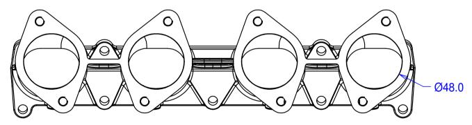
Flanges for Jenvey TB throttle bodies. May be ported up to 52mm. O ring seal to cylinder head Additional material to allow matching to ported cylinder heads Undrilled bosses on underside for idle air / vacumn take off / etc
