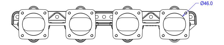
Flanges for Jenvey SF throttle bodies. May be ported up to 50mm at body flange and proportionally at head flange. Option of machined injector pockets.
