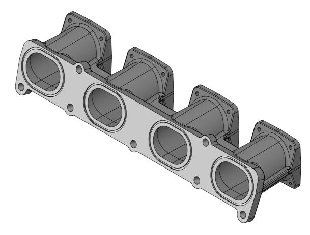
FLANGES FOR JENVEY SF THROTTLE BODIES. FOR SRCC HOMOLOGATED VERSION SEE MF09. UNDRILLED TAPPING BOSSES ON UNDERSIDE OF MANIFOLD FOR BRAKE BOOST, IDLE CONTROL, SENSORS ETC. SEE MF10 FOR LARGER THROTTLE BODY BORES.
