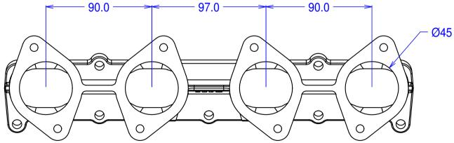
O ring seal to cylinder head Some additional material for porting out Undrilled bosses on underside for idle air / vacumn take off / etc
