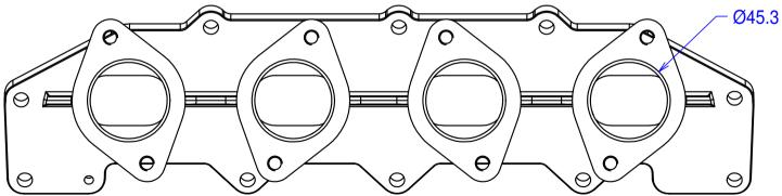
Flanges for Jenvey twin throttle bodies. May be ported up to 50mm at body flange and proportionally at head flange.
