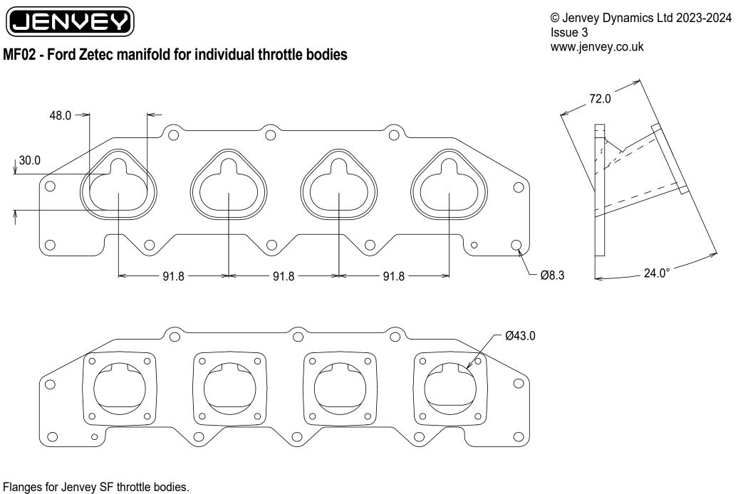
Optional vacuum passage for brakes, fast idle valve, sensors etc. machined in to face. May be ported up to 46mm at body flange and proportionally at head flange.
