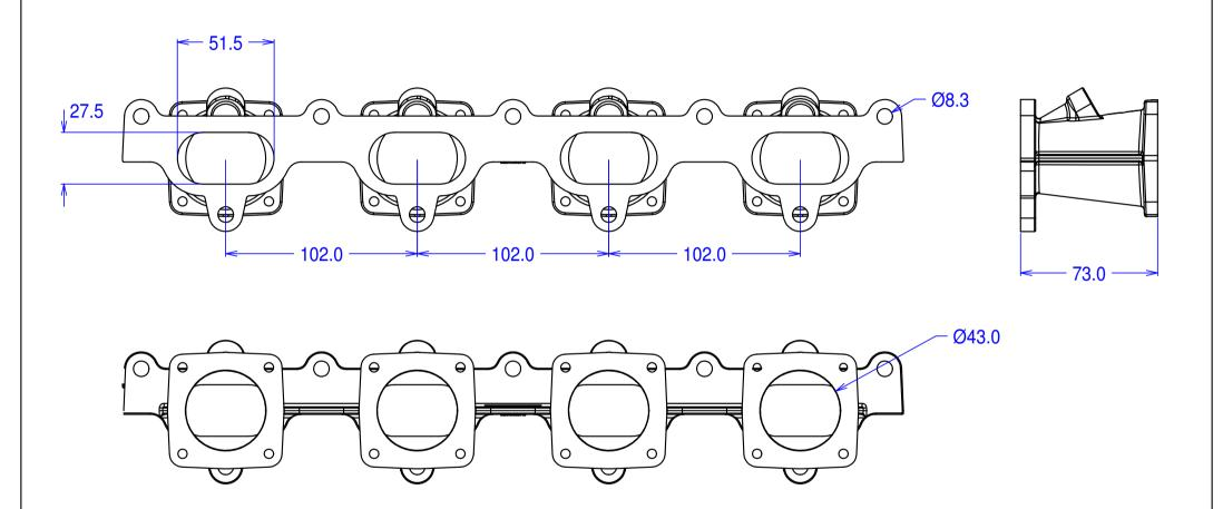
Flanges for Jenvey SF throttle bodies. May be ported up to 50mm at body flange and proportionally at head flange Undrilled bosses on top side for idle air / vacuum take off / injectors / etc.
