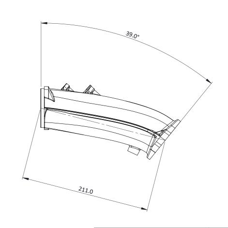
FLANGES FOR JENVEY SSD SPIGOT BODIES, HEAD FLANGE MAY BE PORTED TO SUIT CYLINDER HEAD, BUT NOT THE THROTTLE BODY FLANGE. SUITABLE FOR Ø58mm PARALLEL, OR Ø60mm TAPER BODIES.
