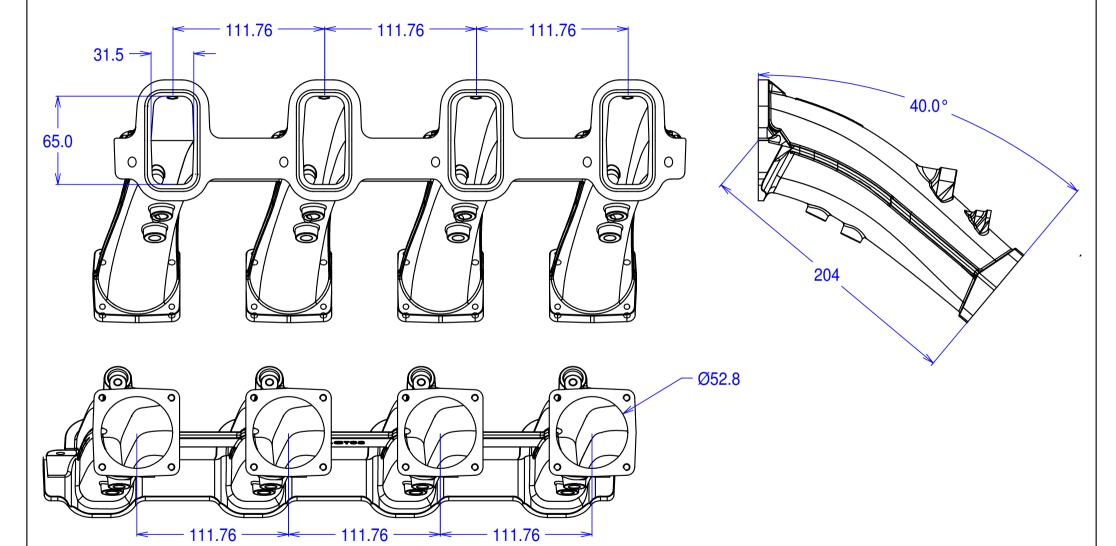
Flanges for Jenvey SFD throttle bodies. Sufficient metal to allow port machining. 'O' ring seal to cylinder head.
