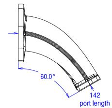
Flanges for Jenvey twin (TB, TH, TS) throttle bodies. May be ported up to 50mm. Additional material to allow matching to ported cylinder heads. Undrilled bosses on underside for idle air / vacumn take off / etc.
