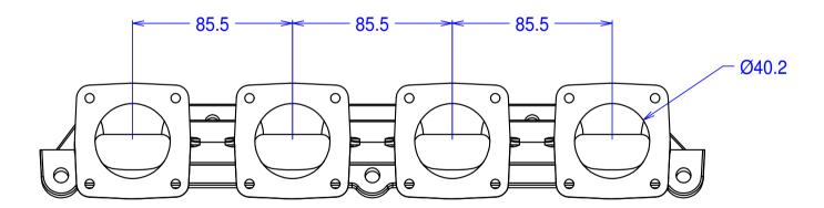
Flanges for Jenvey SF throttle bodies. May be ported up to 45mm at body flange and proportionally at head flange Angled for under-bonnet clearance
