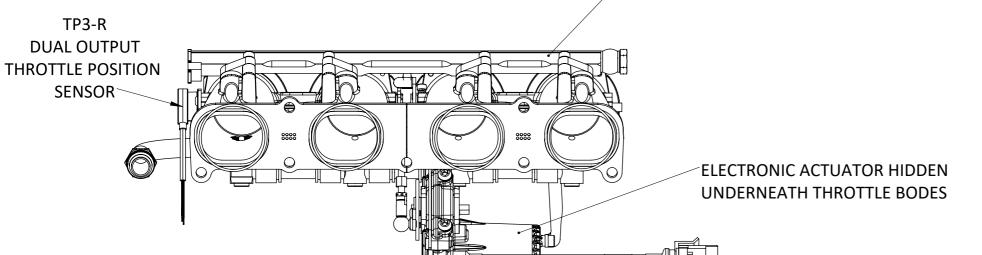
A DIRECT-TO-HEAD THROTTLE BODY KIT TO SUIT THE MAZDA MX5 NC 2.0. THE KIT INLCUDES: Ø45mm DIRECT-TO-HEAD THROTTE BODIES, LIGHTWEIGHT AIRHORNS, ELECTRONIC THROTTLE ACTUATOR, THROTTLE POSITION SENSOR & LOOM TO SUIT STANDARD HARNESS, MAP RAIL AND FITTINGS, POSITIVE CRANKCASE VENT AND EXHAUST GAS RECIRCULATION SYSTEM\*.
