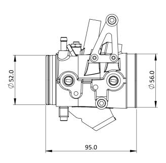
A KIT FOR THE GEN 2 (POST 2008) SUZUKI HAYABUSA ENGINE - USES TWO, TWIN Ø48 BUTTERFLY THROTTLE BODIES WHILST RETAINING THE USAGE OF THE STANDARD FUEL RAIL, INJECTORS, FRONT SPINDLE TPS, REAR SPINDLE ETA MOTOR & TPS, MOUNTING RUBBERS, AIRHORN RUBBERS AND CABLE TRAVEL DISTANCE.
