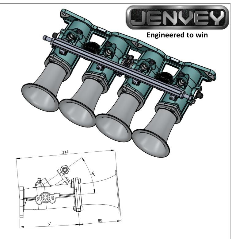
Rover Individual Throttle Body (ITB) kit for fuel injecting your Rover K series engine which contains a linked pair of Ø42mm throttle bodies which attach directly to the cylinder head and four 90mm long air horns. This engine was used in Rover Metro, 200, MGF, Lotus Elise, Caterham and many kit cars. Made to order.
